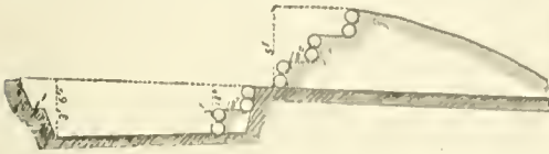
Fig. 2. Profile of a Parallel of a Simple Trench with Steps for Sorties.
